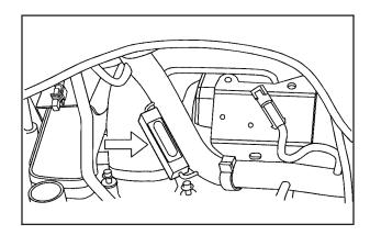
The trailer brake relay is located on the bottom side of the battery harness.
